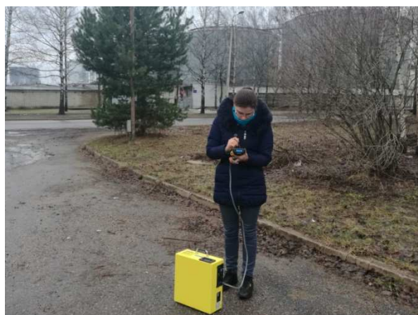
Fig. 2. Field measurements using the Gaset DX-4030 gas analyzer
