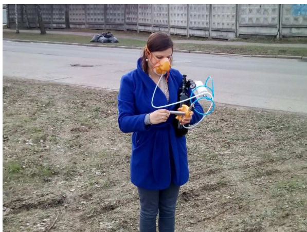
Fig. 1. Field measurements by the Scentroid SM100 field olfactometer
