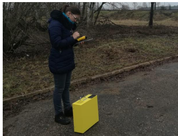
Fig. 2. Field measurements using the Gaset DX-4030 gas analyser
